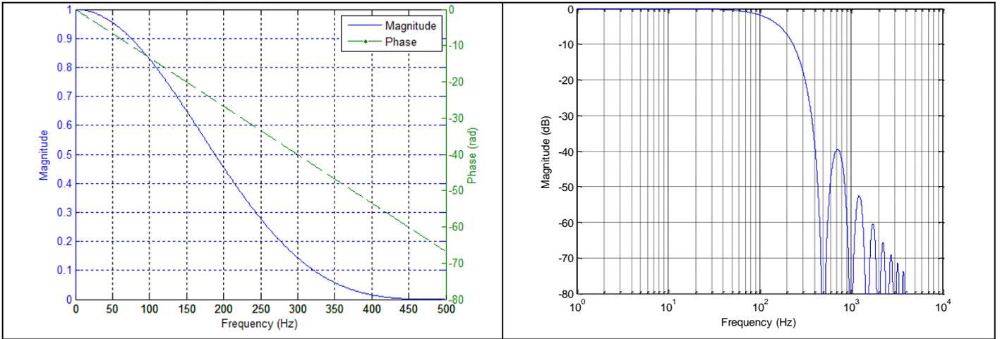
Figure 5-29: Frequency characteristics of AUX with low-pass filter -3dB frequency set to 131Hz
