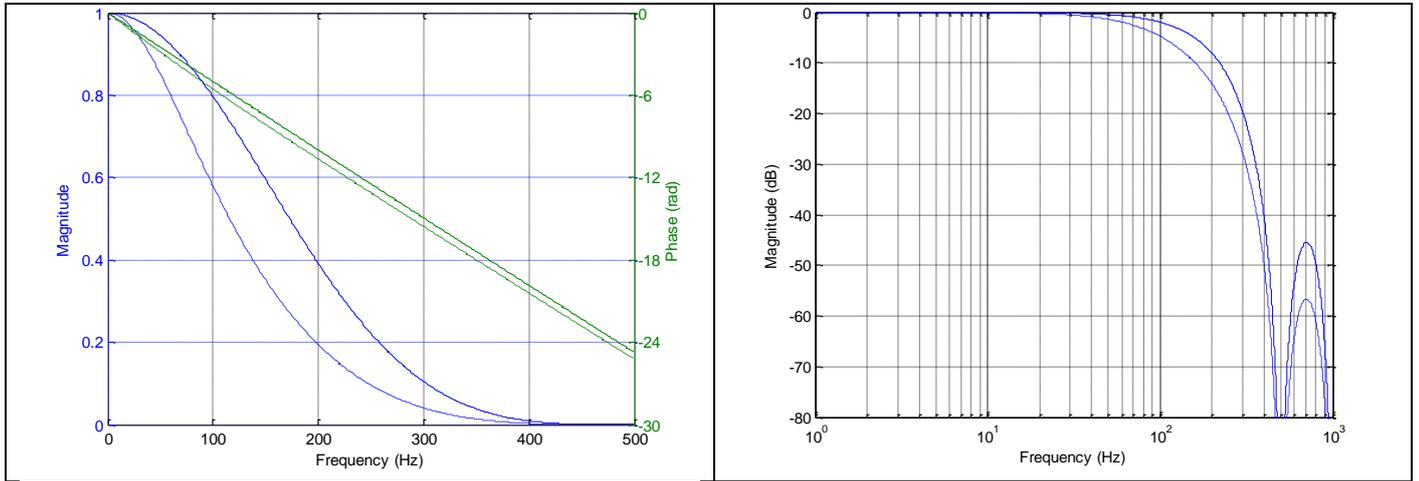
**Figure 5-17: Frequency characteristics of accelerometers with low-pass filter -3dB frequency set to 131Hz (solid line: nominal, dashed line: minimum bandwidth, limited by accelerometer)**
