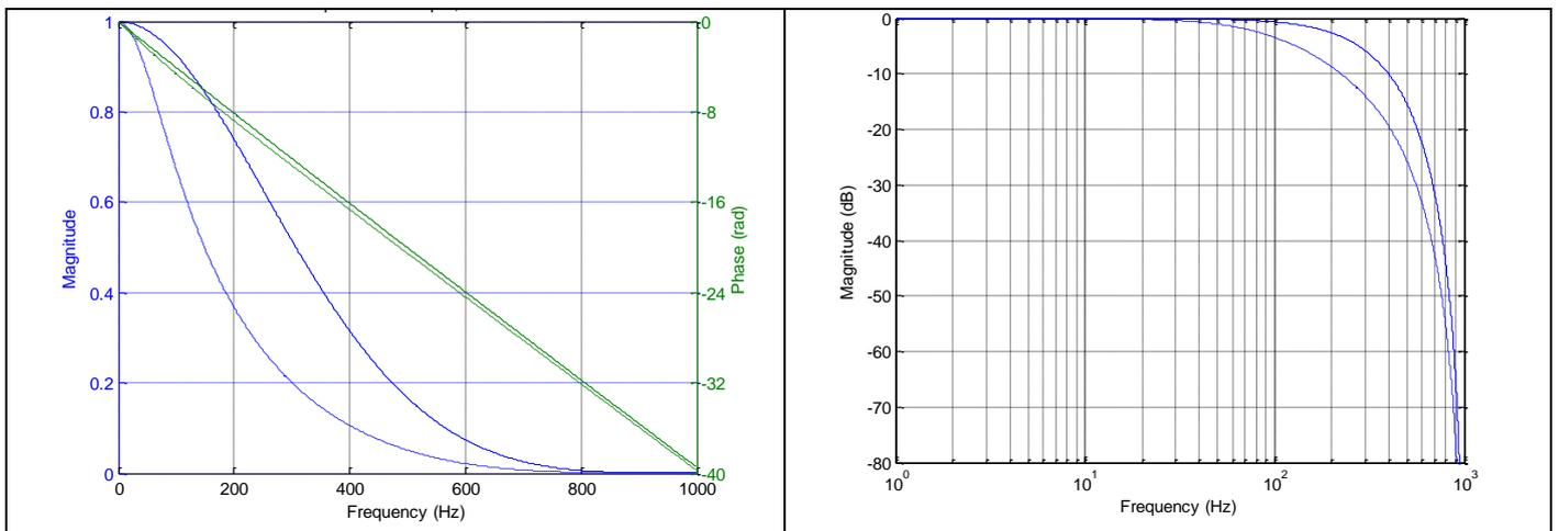
**Figure 5-18: Frequency characteristics of accelerometers with low-pass filter -3dB frequency set to 262Hz (solid line: nominal, dashed line: minimum bandwidth, limited by accelerometer)**
