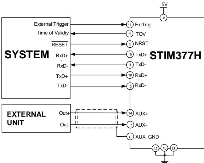
**Figure 7-2: Full Function Electrical Connection Diagram**
