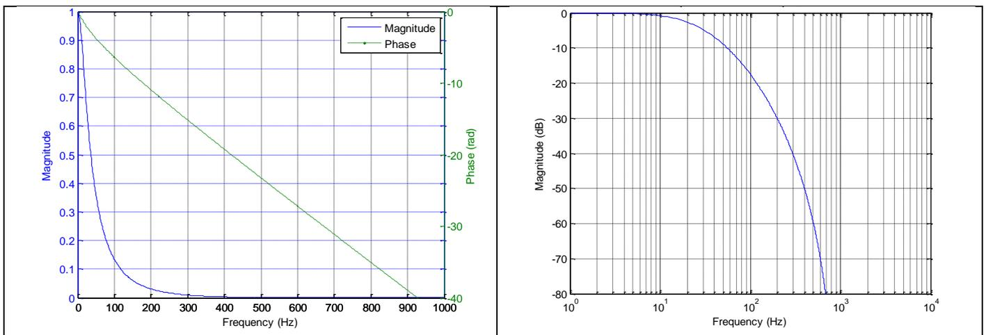
**Figure 5-25: Frequency characteristics of inclinometers with low-pass filter -3dB frequency set to 262Hz**
