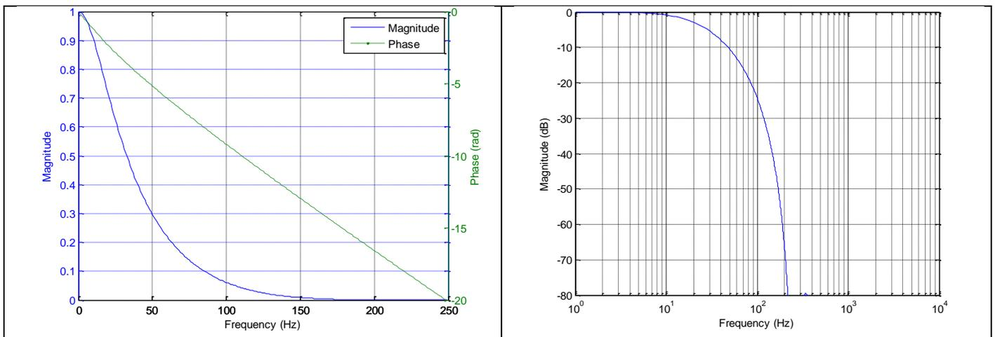
Figure 5-23: Frequency characteristics of inclinometers with low-pass filter -3dB frequency set to 66Hz
