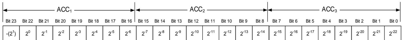
**Figure 7-13: Converting output bytes to [g]**
