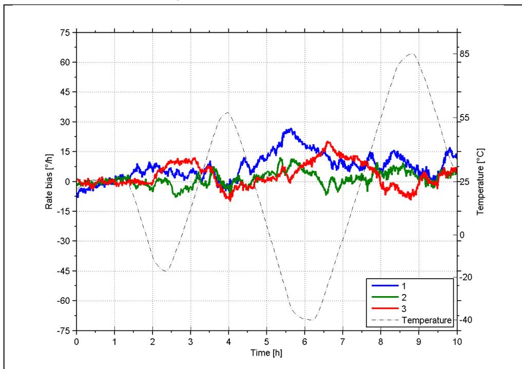
Figure 5-6: Typical Bias drift over temperature (400°/s gyro)
