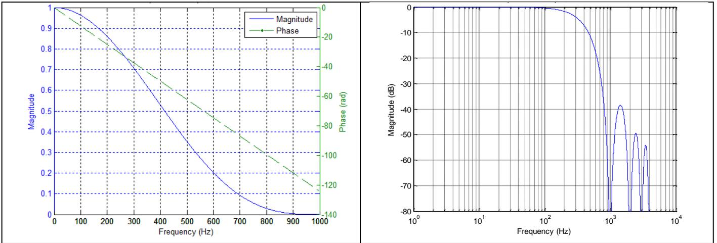
Figure 5-30: Frequency characteristics of AUX with low-pass filter -3dB frequency set to 262Hz
