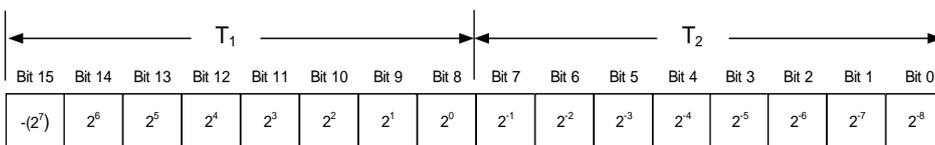
**Figure 7-15: Converting temperature data to [°C]**
