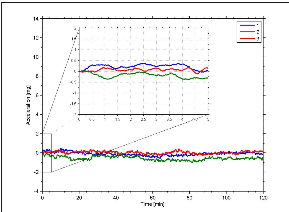
Figure 5-20: Typical normalized initial bias drift of inclinometer
