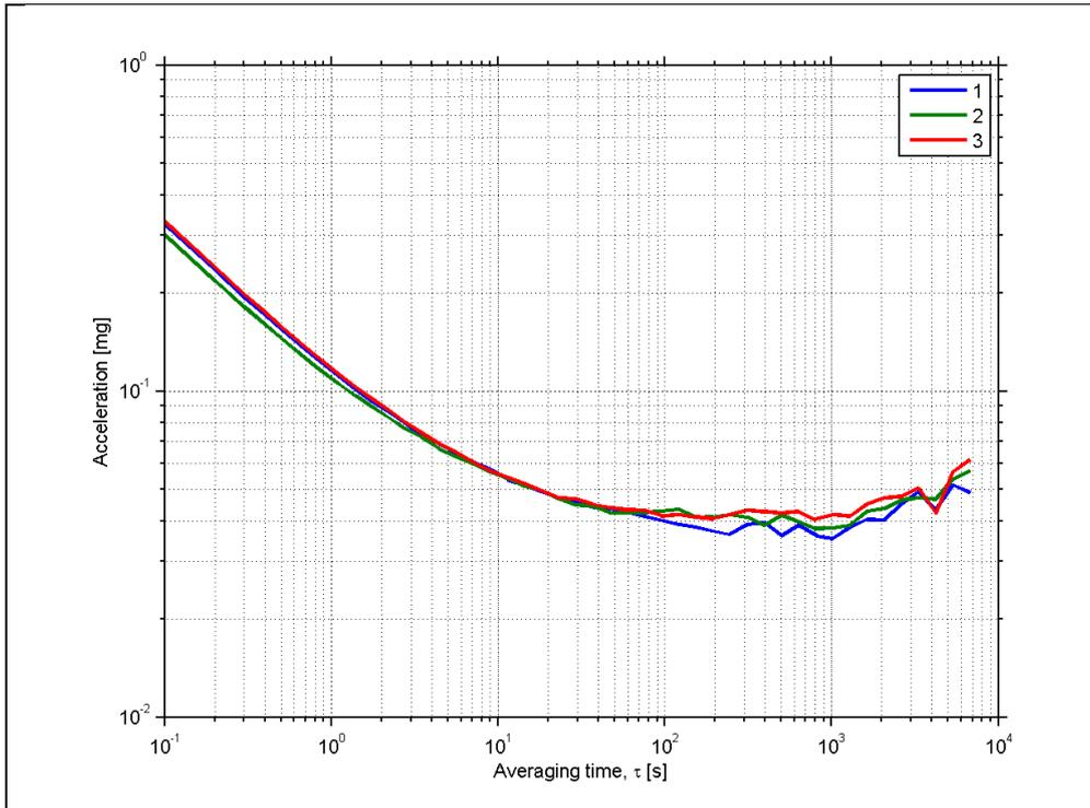
Figure 5-12: Typical Allan-Variance of accelerometer (10g accelerometer)
