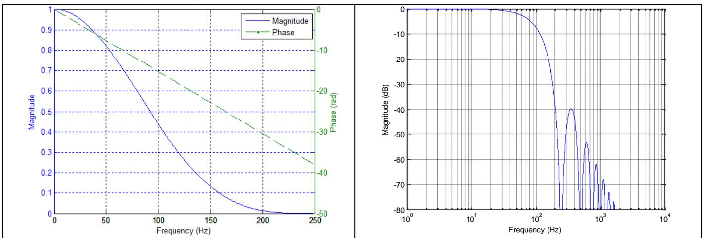
Figure 5-28: Frequency characteristics of AUX with low-pass filter -3dB frequency set to 66Hz
