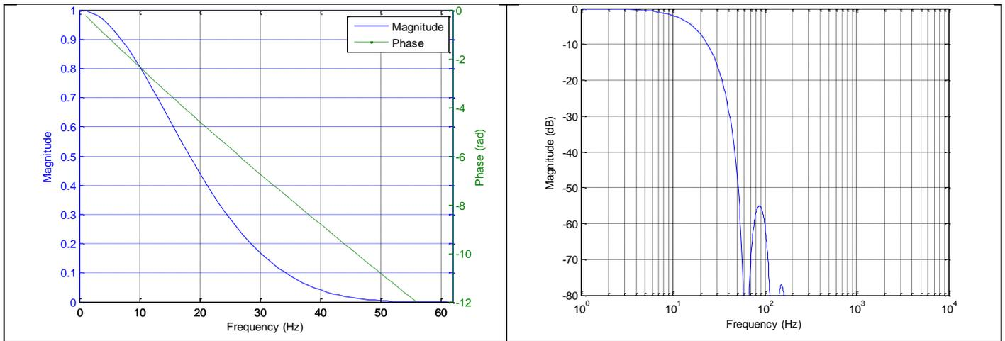
Figure 5-21: Frequency characteristics of inclinometers with low-pass filter -3dB frequency set to 16Hz
