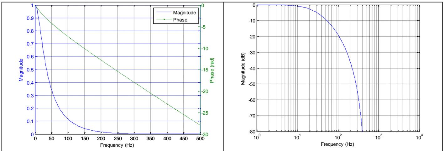
**Figure 5-24: Frequency characteristics of inclinometers with low-pass filter -3dB frequency set to 131Hz**
