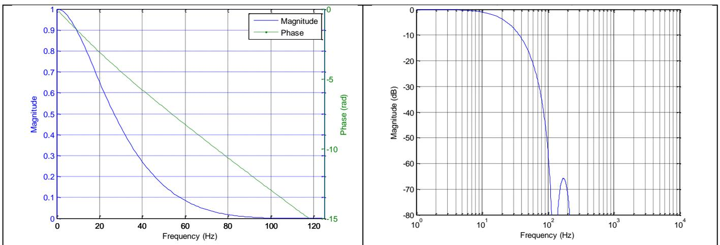
Figure 5-22: Frequency characteristics of inclinometers with low-pass filter -3dB frequency set to 33Hz
