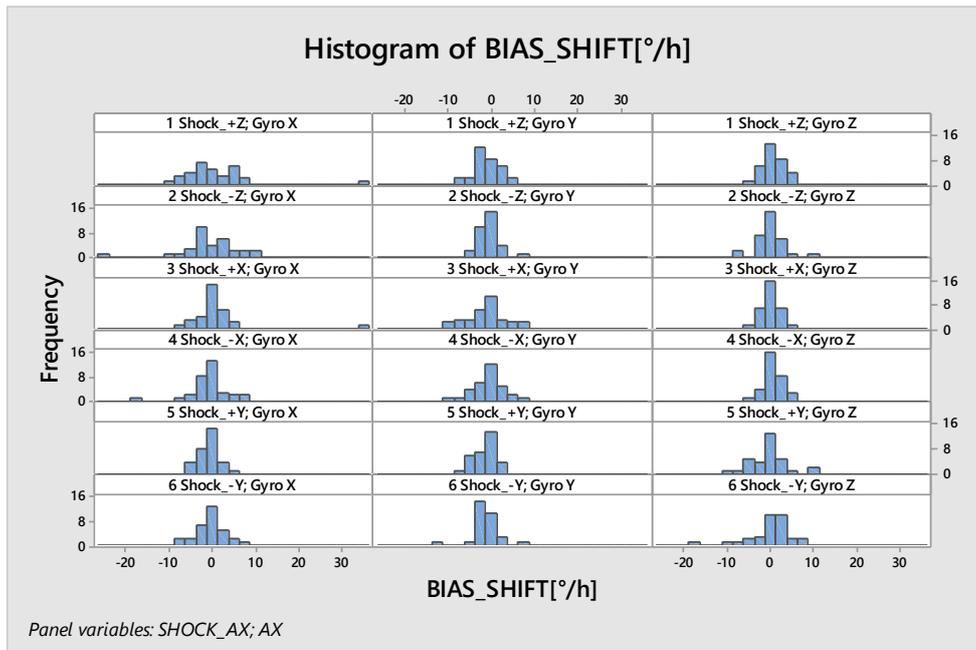
Figure 21: Bias-shifts during shocks in different directions
