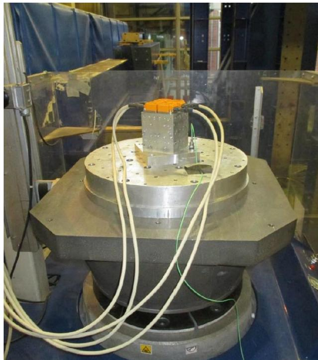
Figure 17: Test set-up for shock tests #3 and #4 (testing in z-direction)
