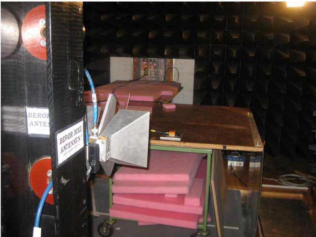
Photo 4.2.4 Test setup regarding RE102, Radiated emissions, electric field.
