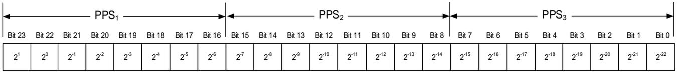
**Figure 7-17: Converting output bytes to [ ]**
