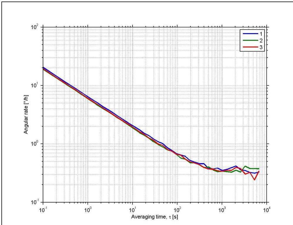
Figure 5-3: Typical Root Allan-Variance of gyro (400°/s gyro)
