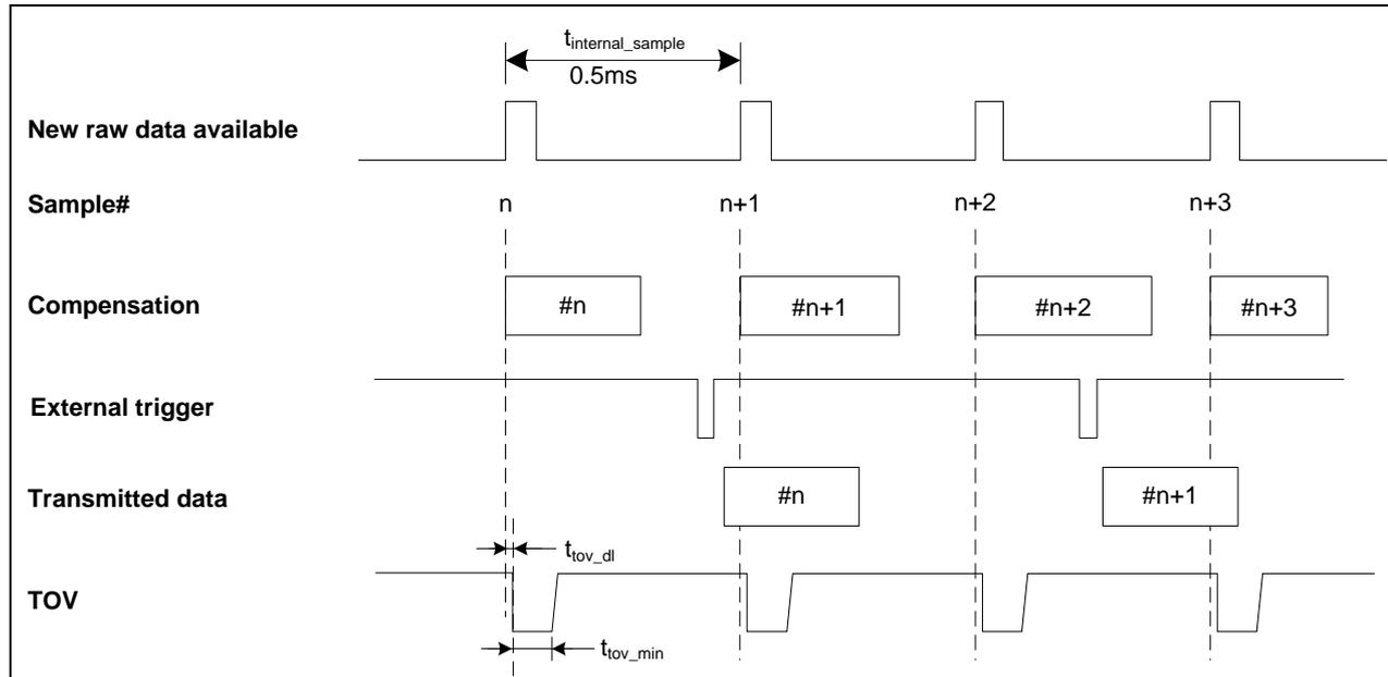
Figure 7-6: Timing of TOV with external trigger
