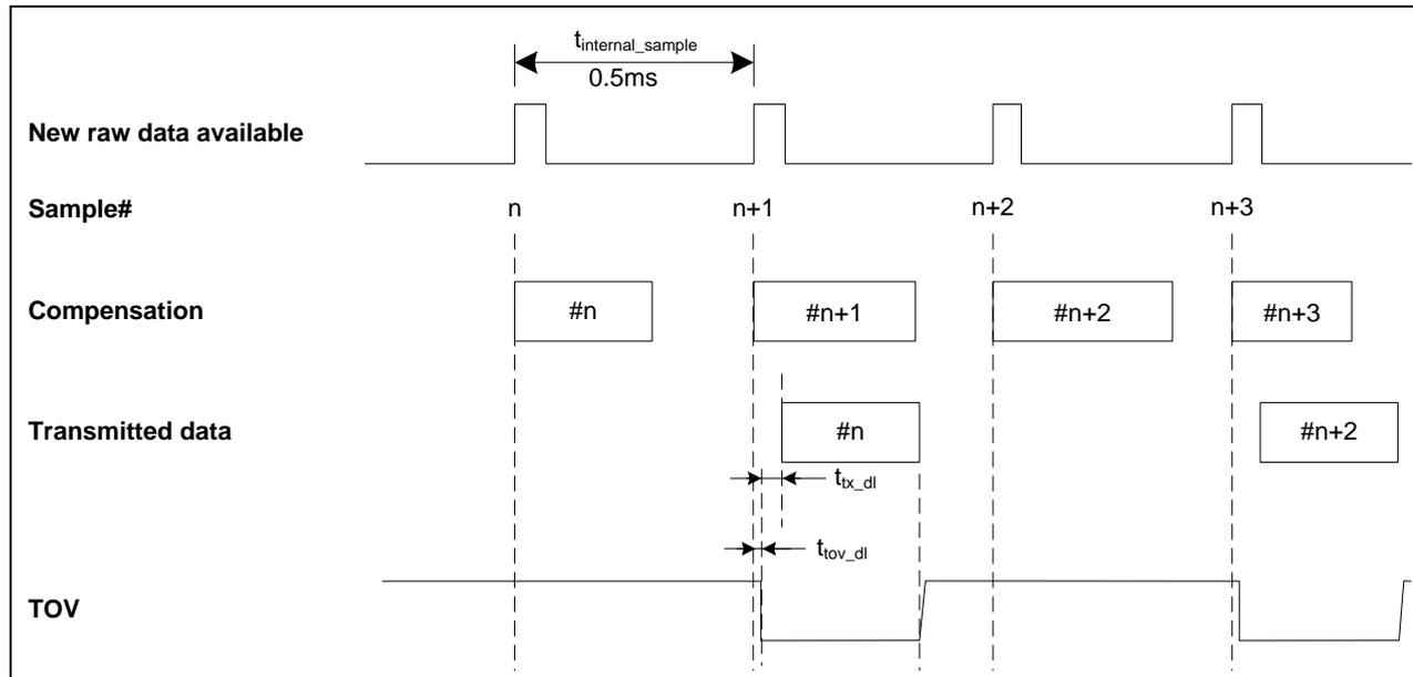
Figure 7-5: Timing of TOV (example: sample rate = 1000samples/s)
