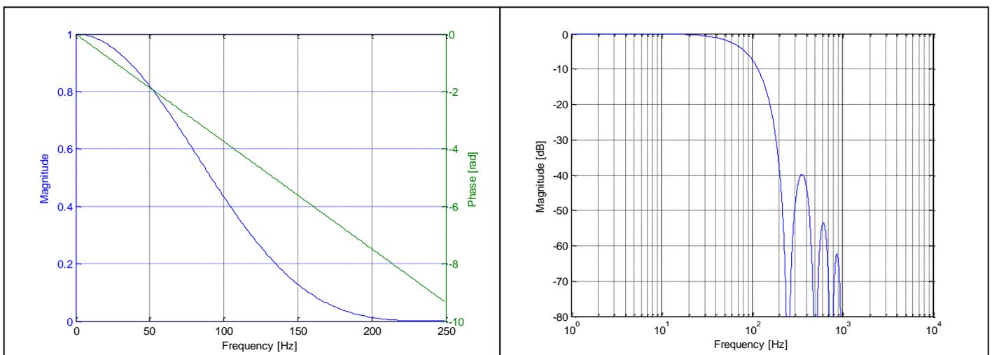
Figure 5-20: Frequency characteristics of PPS filtered with low-pass filter -3dB frequency set to 66Hz
