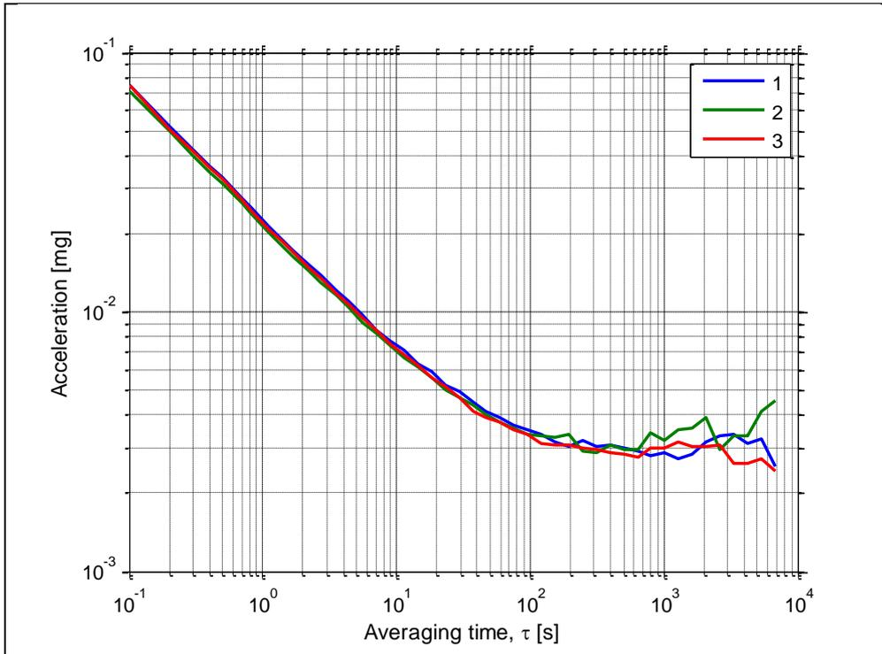
Figure 5-11: Typical Allan-Variance of accelerometer (10g accelerometer)
