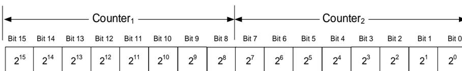
**Figure 7-19: Converting counter to an integer number**
