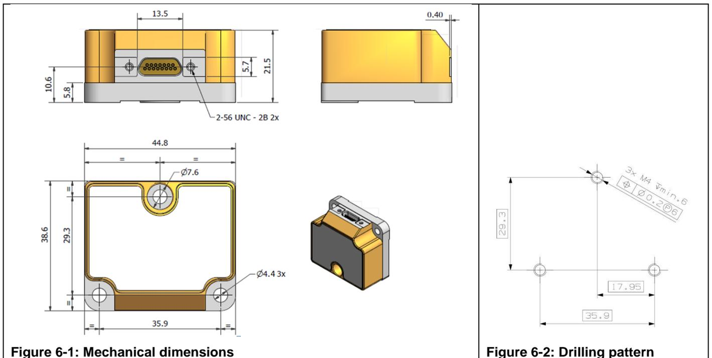
**Figure 6-1: Mechanical dimensions**
