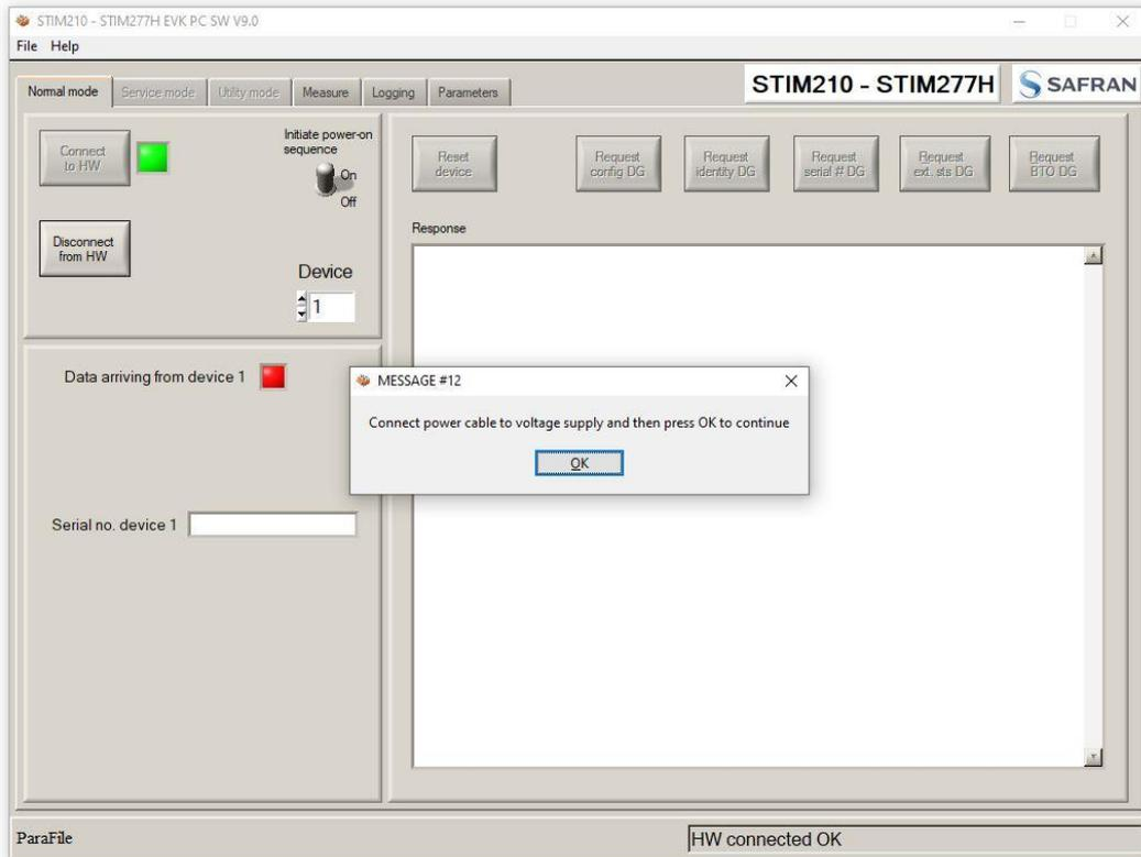
**Figure 20: Confirm power supply is switched on**
