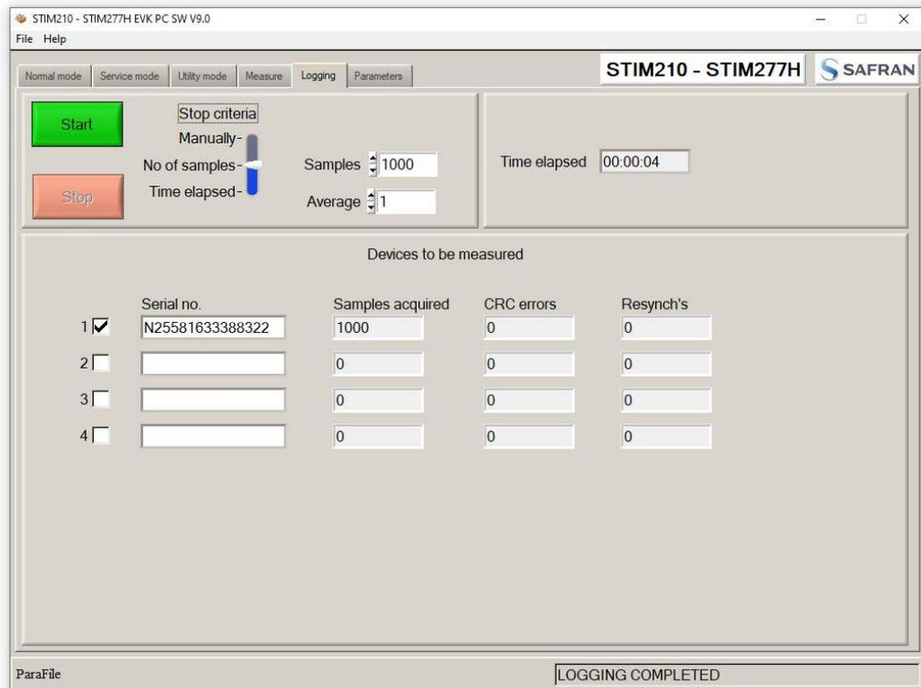
Figure 25: Logging panel (for saving data to file)
