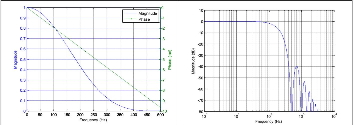
Figure 6-10: Frequency characteristics of gyros with low-pass filter -3dB frequency set to 131Hz
