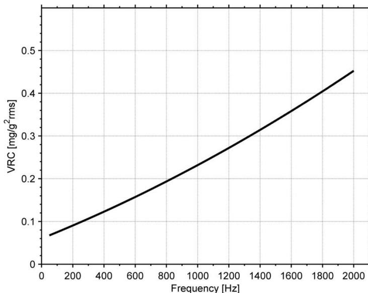
**Figure 6-3: Nominal VRC at 10g rms for 10g accelerometers**
