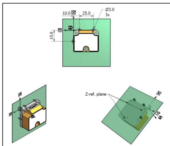
Figure 6-2: Reference points for alignment of axes
