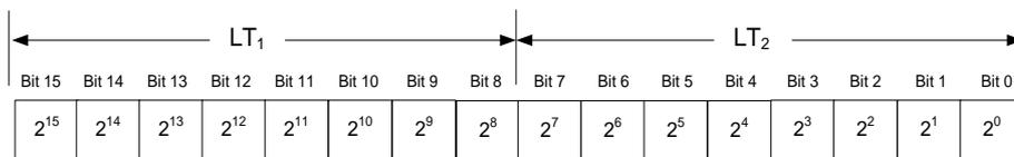
**Figure 8-16: Converting output bytes to [μs]**
