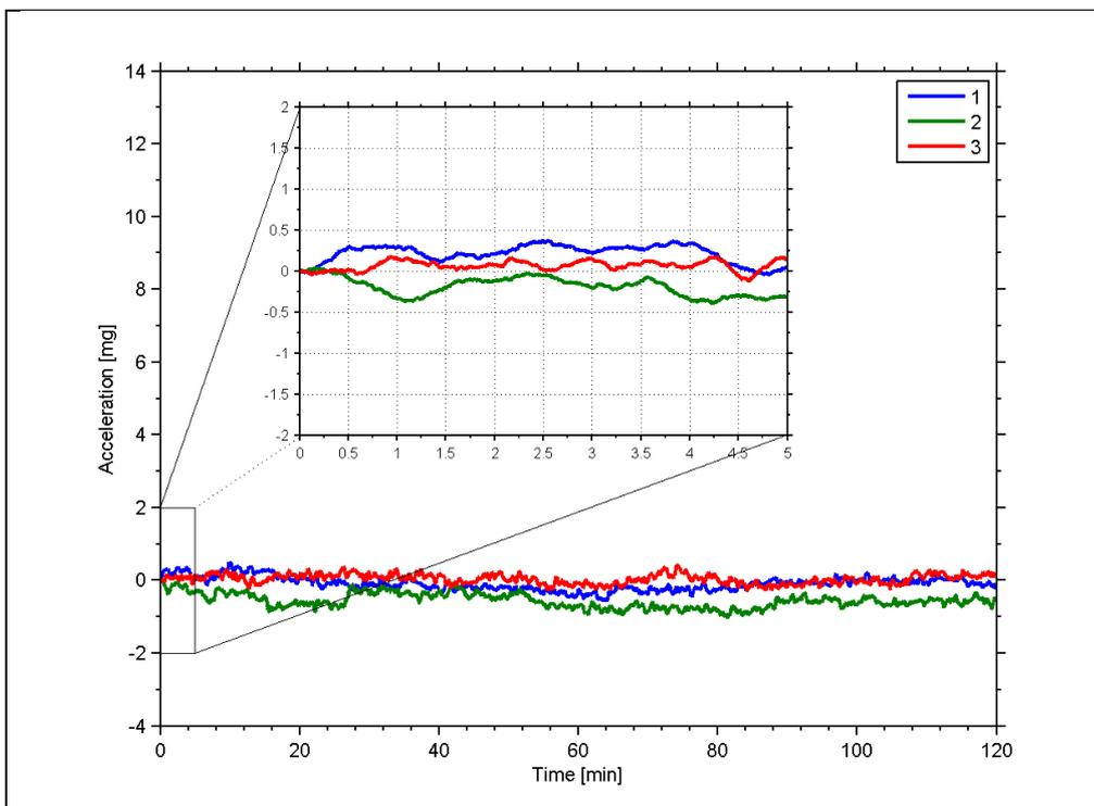
Figure 6-20: Typical normalized initial bias drift of inclinometer
