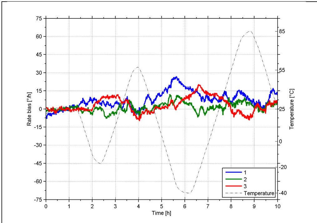
Figure 6-6: Typical Bias drift over temperature (400°/s gyro)
