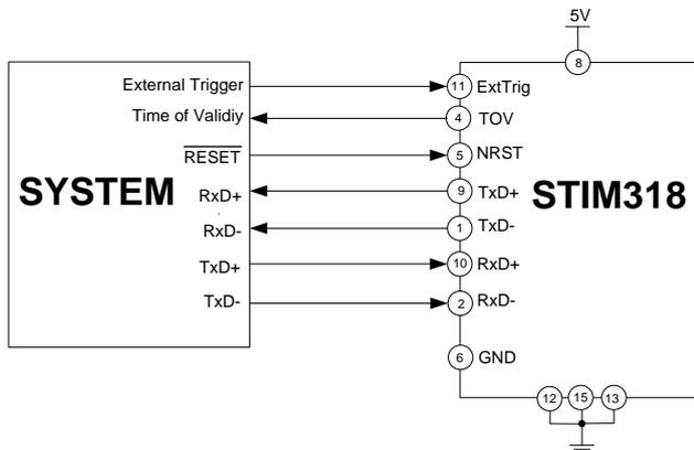
**Figure 8-2: Full Function Electrical Connection Diagram**
