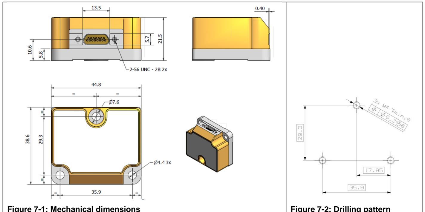
Figure 7-1: Mechanical dimensions
