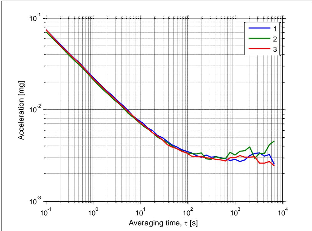
Figure 6-12: Typical Allan-Variance of accelerometer (10g accelerometer)
