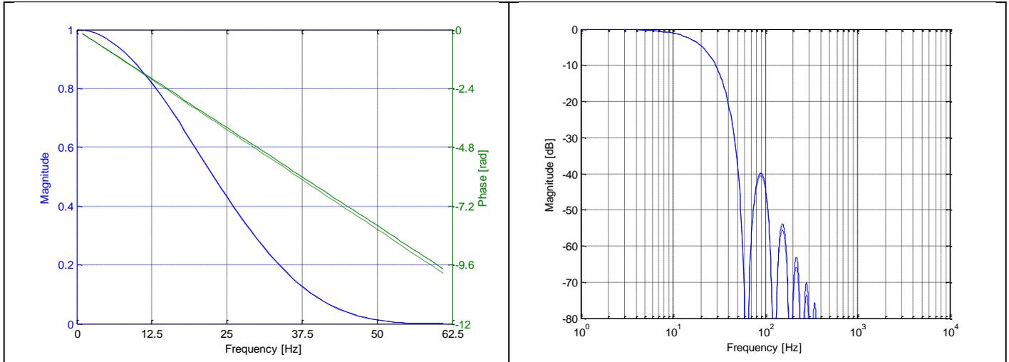
**Figure 6-13: Frequency characteristics of accelerometers with low-pass filter -3dB frequency set to 16Hz (solid line: nominal, dashed line: minimum bandwidth, limited by accelerometer)**
