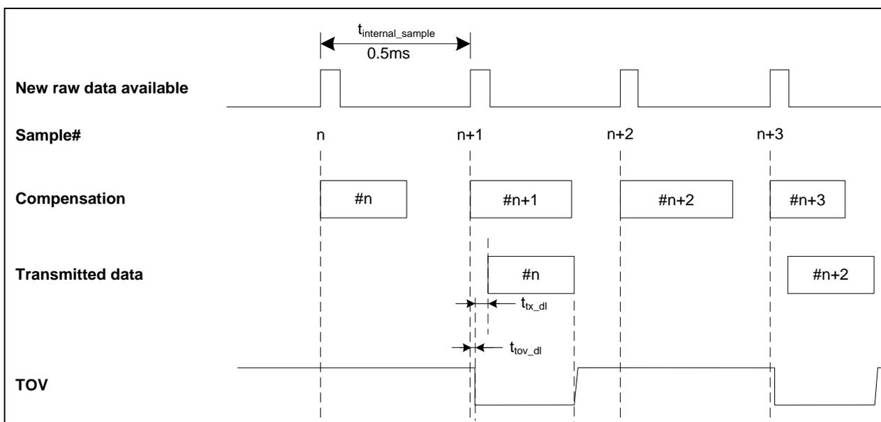
Figure 8-4: Timing of TOV (example: sample rate = 1000samples/s)
