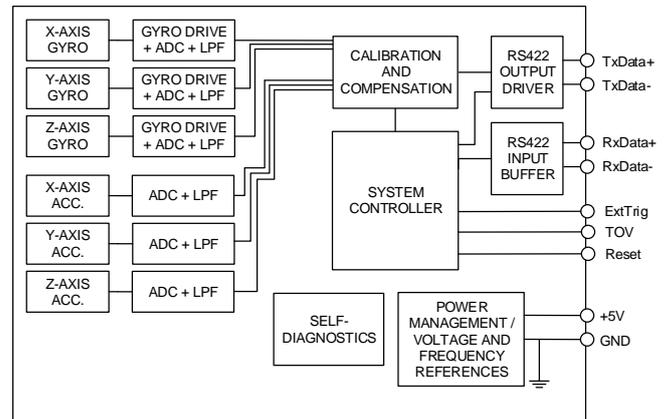
**Figure 2-1: STIM318 FUNCTION BLOCK DIAGRAM**
