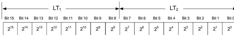
Figure 8-14: Converting output bytes to [ $\mu$ s]
