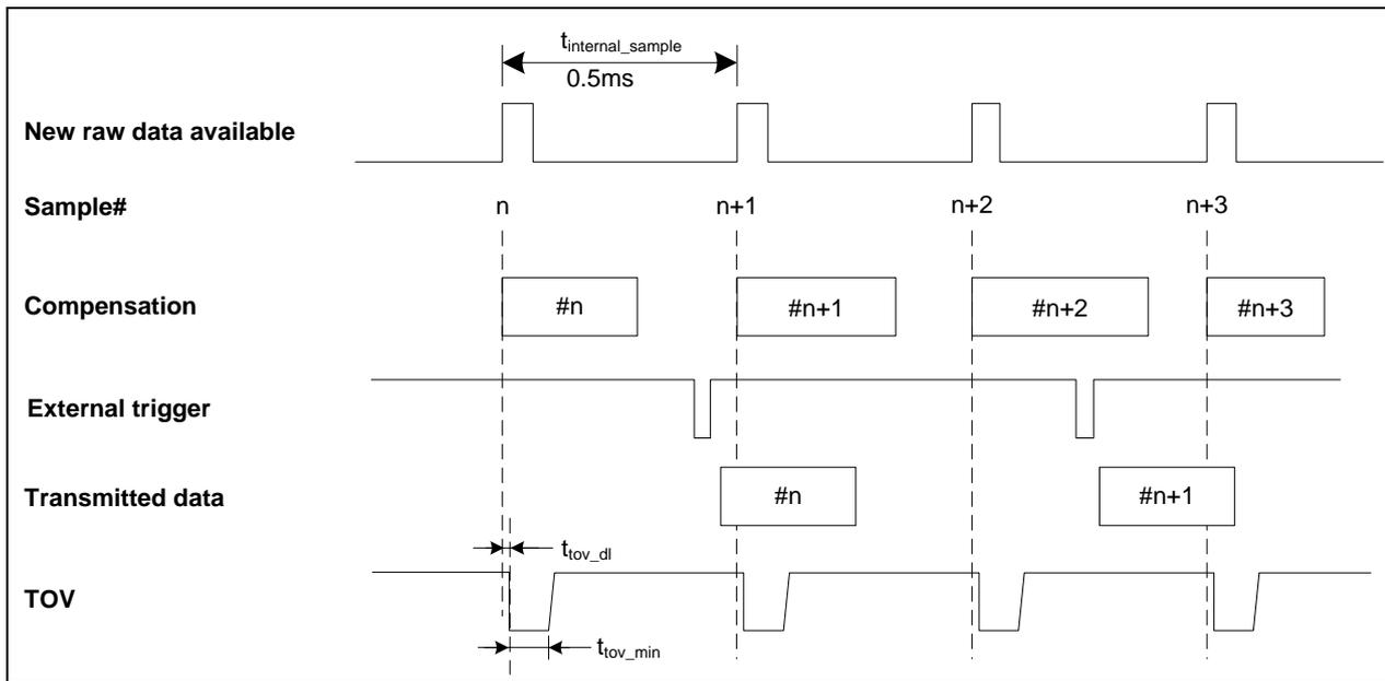
Figure 8-5: Timing of TOV with external trigger
