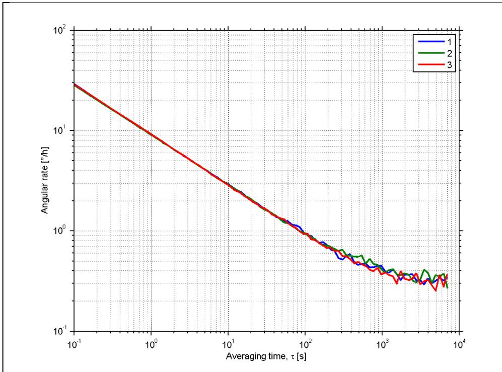
Figure 6-3: Typical Root Allan-Variance of gyro (400°/s gyro)
