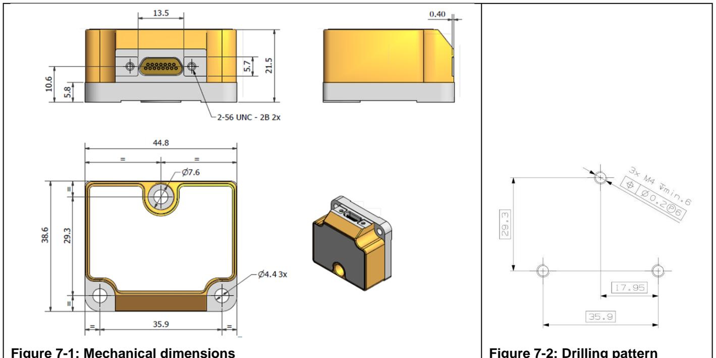
**Figure 7-1: Mechanical dimensions**
