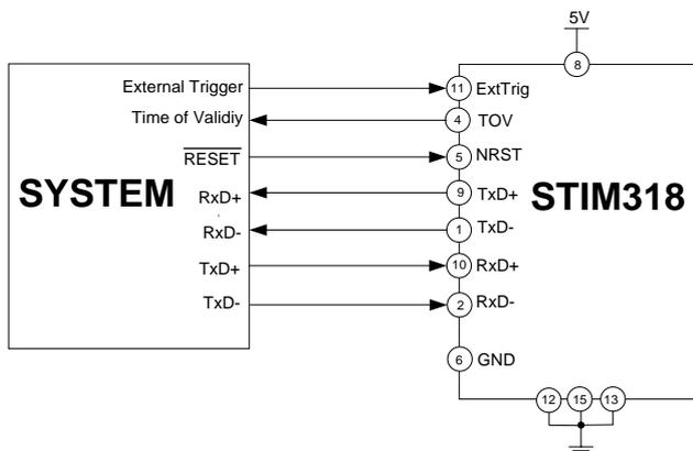
**Figure 8-2: Full Function Electrical Connection Diagram**
